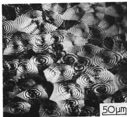
Figure 1 Banded spherulites of polyethylene in a 5 \mu\text{m} section viewed optically between crossed polars and crossed quarter-wave plates
